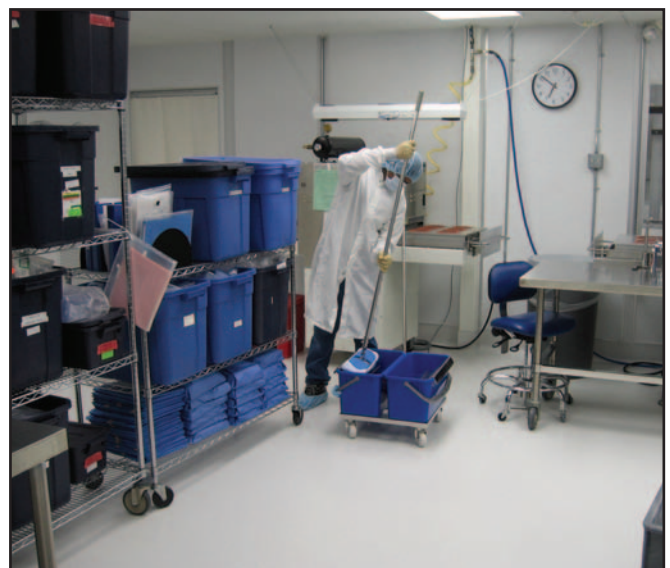
Figure 1: Lint free polyester or PVA mops attached to stainless steel handles are required for mopping.
